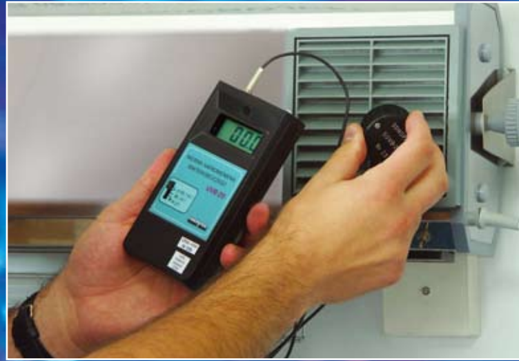
Safe to people – measurement of the irradiation with the use of counter indicates 0
